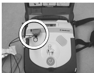
Figure 7. Electrode pad plug (circled) easily becomes detached during use of the Medtronic device.
